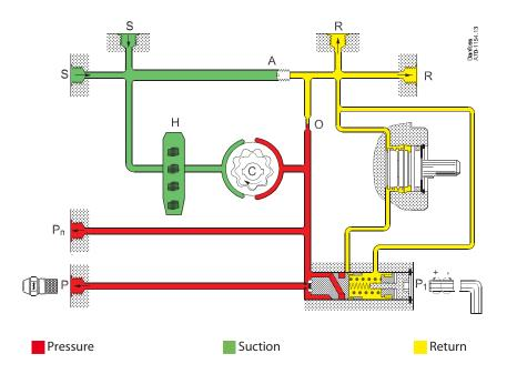
From the suction inlet (S) oil is drawn through the gear set, where the pressure is increased. By means of the piston and the spring in the pressure regulator the pressure is kept constant at the value set on adjustment screw  $(P_1)$ .
