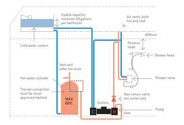
CT pump range twin ended positive head with up and over pipework and natural flow of  $1 \mbox{Litre/min}$  per side.
