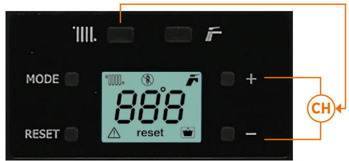
Figure 4.3. Setting Flow Temperature
