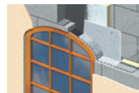
Parabolic Arch lintel
